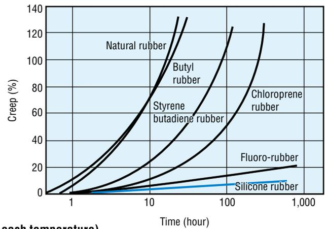
\* Creep is the deformation of a plastic material under constant load. Typically, creep increases as temperature rises. Rubbers that are firm and have greater thermal stability tend to exhibit lower creep values at higher temperatures. Silicone rubber exhibits less creep than organic rubbers, and is more stable even than fluoro-rubber, which has good heat resistance.
