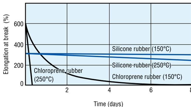
Chloroprene rubber deteriorates rapidly and discolors at temperatures between 150°–250°C, but there is little change in silicone rubber even at 250°C.
